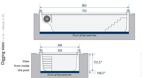
Needed for unloading & placing the pool **CRANE** 13 tons  $^{st}$  Depth taken from under the coping stone
